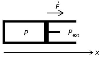
$$\begin{aligned} \sum \vec{F} &= F \vec{e}_x + SP \vec{e}_x - SP_{\text{ext}} \vec{e}_x = \vec{0} \\ \Rightarrow P_{\text{ext}} &= P + \frac{F}{S}, \end{aligned}$$
