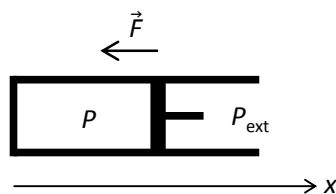
$$\begin{aligned} \sum \vec{F} &= -F\vec{e}_x + SP\vec{e}_x - SP_{\text{ext}}\vec{e}_x = \vec{0} \\ \Rightarrow -F + SP - SP_{\text{ext}} &= 0 \\ \Rightarrow P_{\text{ext}} &= P - \frac{F}{S}, \end{aligned}$$
